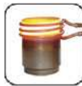
Annealing of S.S. tube
